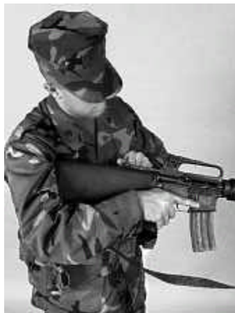
Figure 7-1. Pulling Charging Handle with Left Hand.
